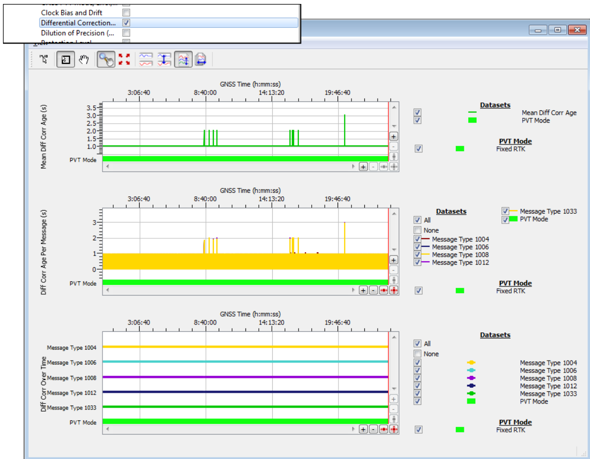
Figure 5-10: Time plot of RTCMv3 differential correction reception
