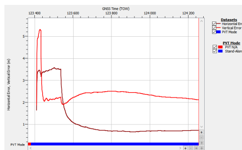
Figure 5-24: Position Error time plot
